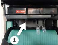
Check if the mixing tray (1) is present, and/or full inserted into the machine.
