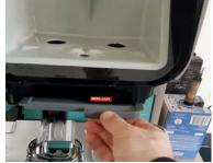
Slide the mixer tray back into the machine. If necessary, exercise a little pressure to ensure it is fully inserted.
