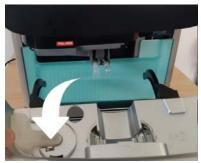
If the panel does not hinge smoothly: Remove the panel entirely. (Hinge down and pull towards you)
