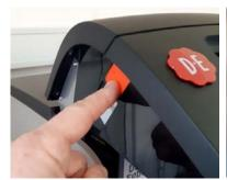
Press the [standby] button for 5 seconds to reset the machine. The button is located at the left side of the door. (Open the door to reach)
