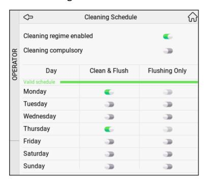
In the Cleaning Day menu you can adjust the day(s) that the dispenser will automatically request to be cleaned by selecting Yes for automatic request on that day, or No to prevent cleaning request on that day.
