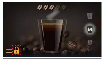
1. When the LOCK icon is displayed on the screen, the drink delivery is blocked. The cooling compartment and the boiler will remain in operation. Press the LOCK icon to unlock the machine.
