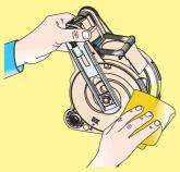
Dry the parts accurately: head of mixers, exhaust system parts, funnell for coffee powder and brewer.
