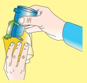
Dry the drip tray for nozzles, head of mixers, exhaust system parts.
