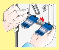
Unscrew the knurl and remove the frontal bar.
