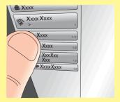
For rinsing: close the door (or simulate door closing by placing the yellow key into its slot) select "Wittenborg" then "Maintenance" and "Daily operations".
