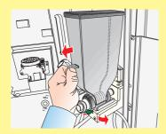
Remove sugar canister: turn it up pull it outward then press the green lever below. Put it on a talble
