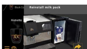
Put the milk pack back into the fridge, and insert the milk supply tube into the pack.
