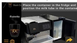
Place the container with cleaning solution in the fridge and place the milk tube in the container.
