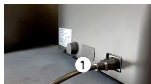
Connect the power cord (1) to the machine, and plug into a power outlet.
