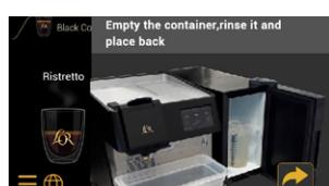
Empty the container. Rinse, and place back. The machine will continue the cleaning program.
