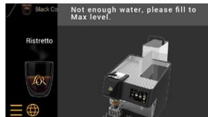
If there is not enough water in the water tank during the descaling process, a display message will prompt you to refill the water tank.
