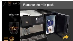
Remove the milk pack from the refrigerator. Check the 'best before date' and replace if necessary.
