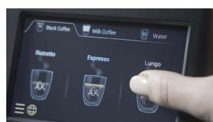
Press the lungo or cappuccino (for coffee-milk machines) selection button. **(Do not put a coffee disc in the machine.)**
