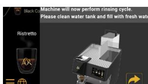
The machine will thereafter perform a rinsing cycle. Please clean the water tank and fill with fresh water. Re-install the water filter from the tank if applicable.
