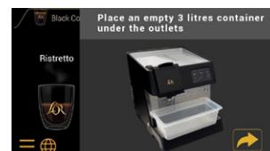
Place an empty 3 litre container under the outlets.
